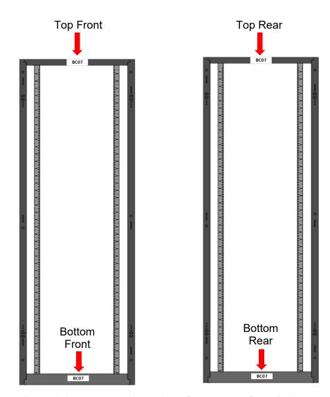
Place labels at the top and bottom, both front and rear of racks/cabinets
