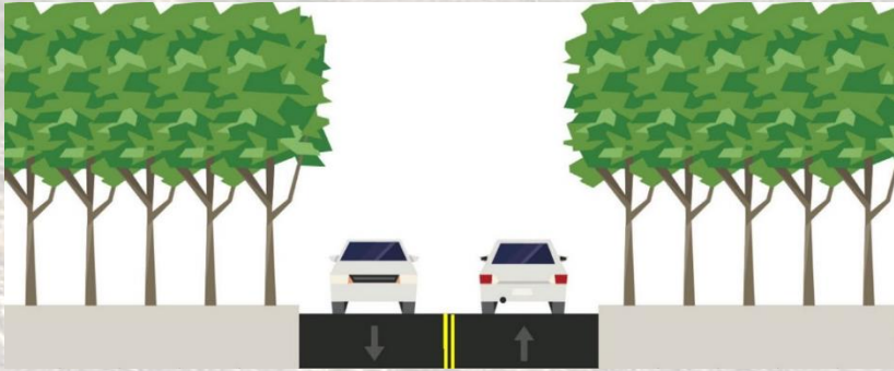
Narrowest Roadway Concept: 20-foot wide with 10-foot lanes, no shoulders
