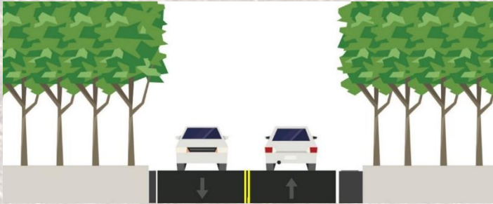
24-foot roadway with 10-foot lanes and a 1-foot shoulder and 3-foot shoulder
