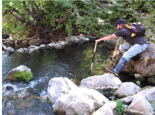
Figure 4.1 Measuring pool depth for habitat function.
