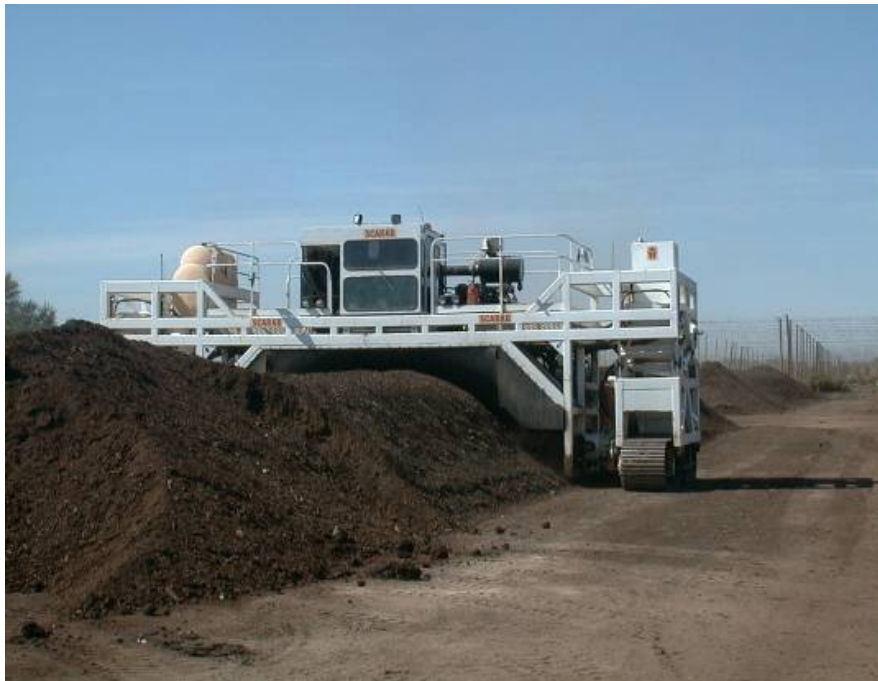
Figure 4-15 Example of Windrow Compost Pile Being Turned
