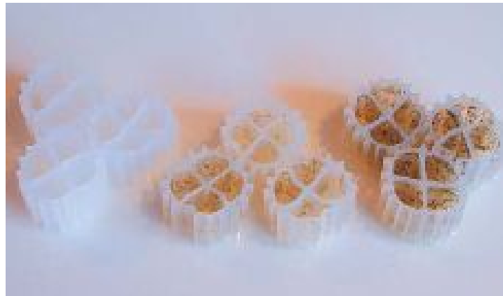
Figure 4-5 Photo of Kaldnes Suspended IFAS Media Showing New Media On Left and Media with Biogrowth On Right
